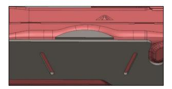
Fully weld frame plates. Don't just burn 1 entire plate, jump from one side to the other, and front to back. Welding no more than 6" at a time. Once fully welded, grind the outer faces of the frame sleeves smooth, the steering boxes need to sit flat up against the frame. (Picture below has all 7 holes installed for reference only)
