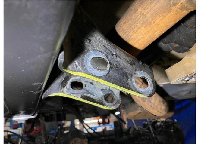
13. On the Passenger side of a **JL**, you will re-use the factory M12x1.5 bolts and supplied M12x1.5 Nylock Nuts, leave loose. See **Fig. O**.
