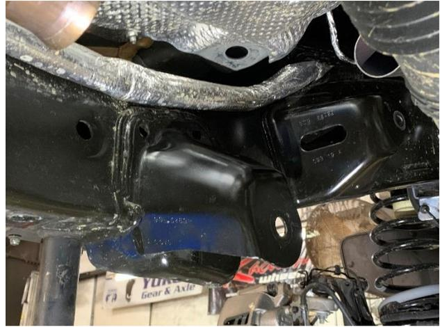
6. On some models of the JT Gladiator, you also need to remove the factory tube stud that's welded to the inside of the frame.
