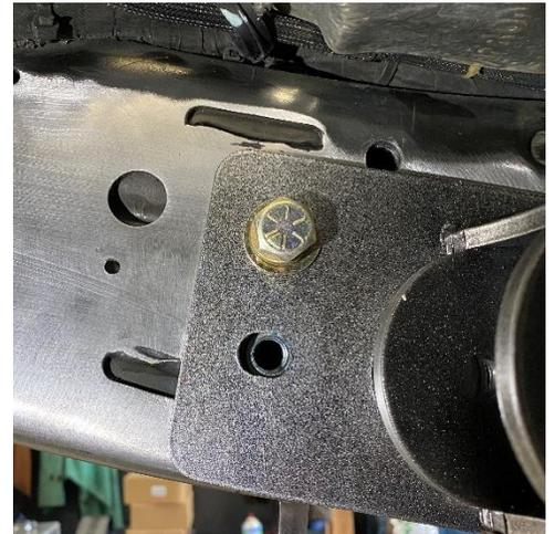
20. If your JL or JT does not have a Preventive Rollover Plate, you will use the other T shaped 2 nut plate. This dual nut plate will go in the hole just under the front body mount. **Fig. W**
