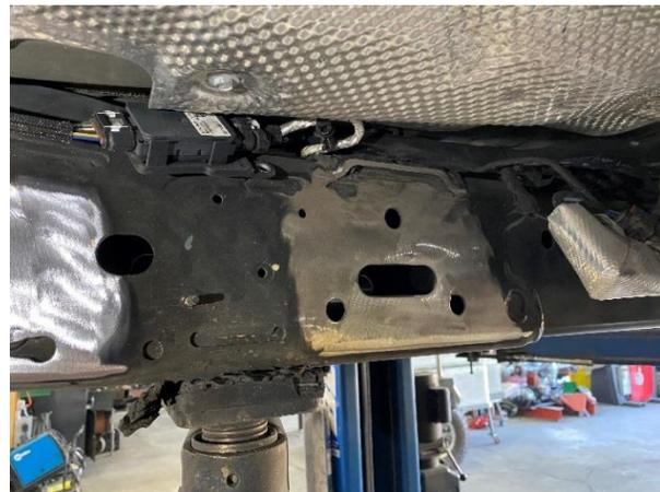
9. Once all brackets are removed, grind clean, and touch up with a semi flat black paint **Fig. L**
