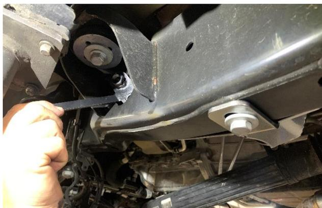
21. Using one of the single nut plates with an angled tail, the nut plate will go through the oval hole on the outside of the frame rail between the link mount and crossmember. See **Fig. X**. All will use ½"-13x1.75" G8 bolt, Lock Washer, and Washer
