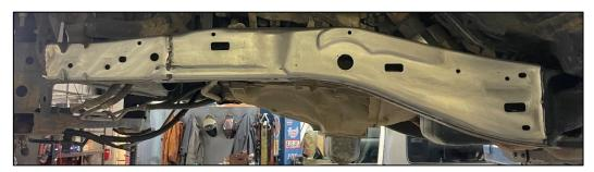
Once both sides are clean and prepped, locate the Driverside inner and outer frame plates. One of the 7 holes will locate on 1 of the holes in the frame. The 2 pictures below show the hole referenced. It's roughly 7-5/8" back from the body mount. Position and clamp frame plate to frame with a few C-clamps.
