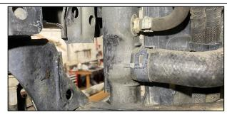
Once the steering box of your choice bolts up without bind, you can remove and tack the frame plate on. We recommend tacking it about every 6" - 8" around the perimeter. Repeat with the opposite side. Supplied with the plates are 2 curved pieces. These go in the divot which was where the strut tower was. Refer to the pictures below on where to place it.
