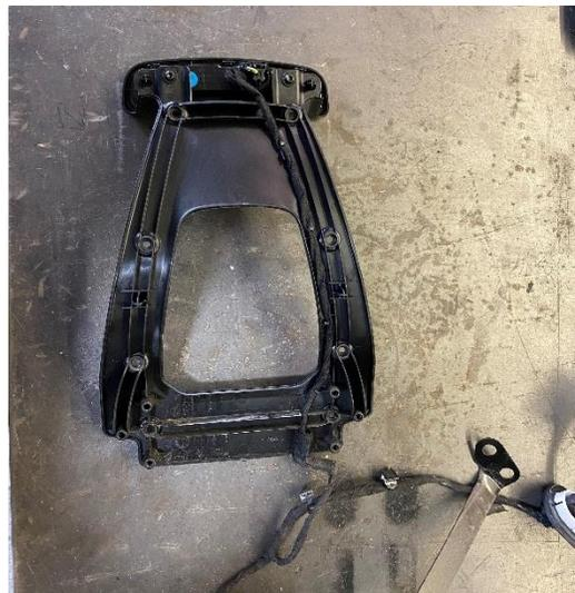
7. Finally, remove the harness from the camera. Using a T-20, unscrew the clip that retains the camera in the housing. (Fig J) Completely remove and set aside for install. (Fig K)
