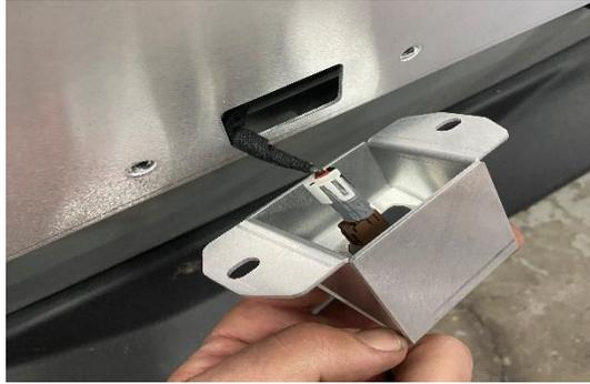
11. If you purchased our 3<sup>rd</sup> brake light kit, follow the instructions that come with them to identify the correct colors. You will use the previously removed 3<sup>rd</sup> brake light wire harness that you rerouted through the vent with the camera wire. You will need to snip the connector off to use these wires.
