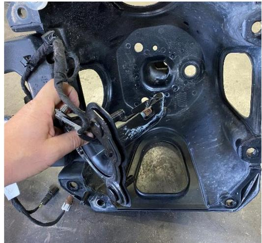
6. Next, you'll need to remove the harness from the 3<sup>rd</sup> Brake light housing. With a T-30 remove the 4 screws from the front side. Then a T-25 to remove the remaining 8 screws. (Fig. H) Pry the plastic housing apart and un-clip the plug from the 3<sup>rd</sup> brake light. Un-clip any remaining retainers and set the light and hosing aside. (Fig. I)
