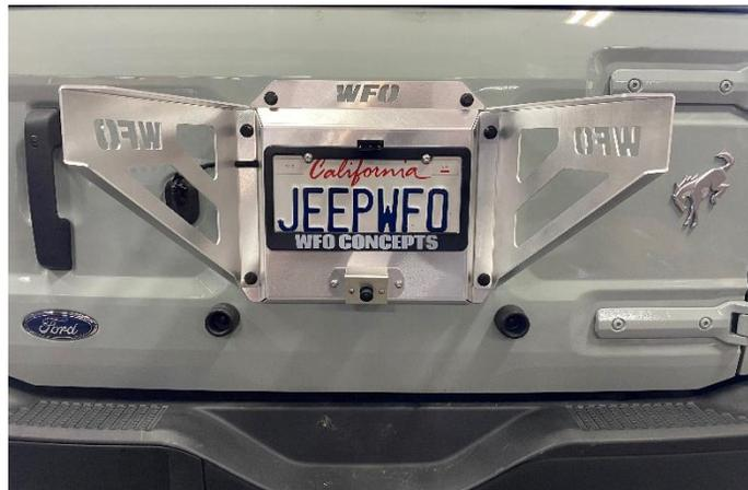
14. Locate your WFO 1401 Basket. If you have not previously assembled the basket, refer to those directions for assembly. Place the basket on the support wings. You will use Qty. (4) holes only. Look at the below picture for the holes. Fig. Q. Align the basket with the support wings till all 4 line up. You will use Qty (4) ¼"-20 x ¾" Button Allens, Qty. (8) ¼" SS Washers, and Qty. (4) ¼"-20 SS Nylock nuts.
