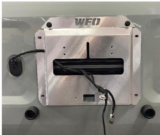
9. Take all 3 camera mount pieces. Start by sliding the pinch plate over the camera, with the Pem nuts facing away from the lens of the camera. Fig. M. Place the camera in the main mount, make sure the wire plug is pointing down out of the bracket. Slip the outer cover over everything. And last take the Qty. (2) #10-32 Button head allen's and thread them into the pinch ring. Fig. N
