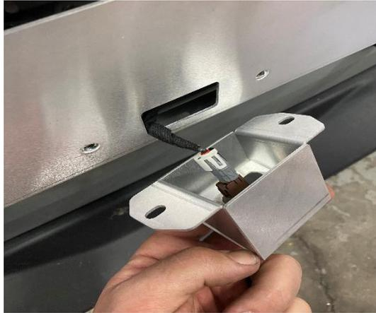
11. If you purchased our 3<sup>rd</sup> brake light kit, follow the instructions that come with them to identify the correct colors. You will use the previously removed 3<sup>rd</sup> brake light wire harness that you rerouted through the vent with the camera wire. You will need to snip the connector off to use these wires.
