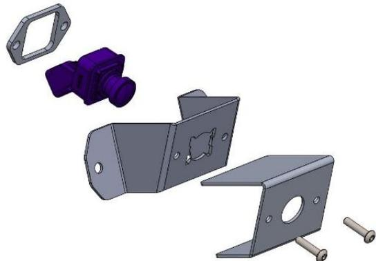
10. Connect the camera plug back onto the camera. Use qty. (2) ¼"-20 x 5/8" Button allen's and bolt the camera onto the license plate mount. Fig. O
