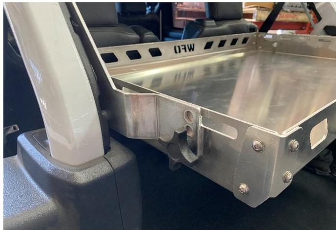
10. Tighten all 4 thumb screws and load up your new basket!
