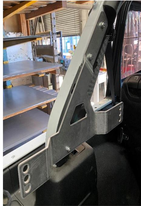
9. Locate the 4 ½"-13 thumb knobs and the previously assembled WFO 1400 Aluminum Basket. Use assistance to hold the basket up between the previously installed brackets and thread the knobs in at the desired height. Each set of holes is ¾", totaling 1-1/2" overall adjustment. See **Fig. G**
