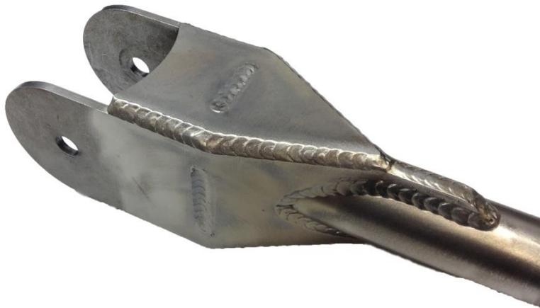
**NOTE: When installing the clevis arms on the axle, the caps will be opposite of each other. For instance, the upper links should have the cap on the top side and the lower links will have the cap on the bottom side. This is for clearance issues with the factory axle bracket during cycling of the suspension. Otherwise, the clevis arms will hit the factory axle bracket.**
