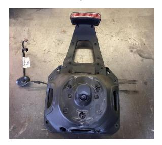
5. Remove the 2 bolts, Socket T-30, on either side of the camera mount (Figure F). This will allow you to remove the bracket from the inside of the spare tire mount. Flip over and gently pry the bracket up from the inside out. (Figure G)
