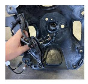
6. Next, you'll need to remove the harness from the 3<sup>rd</sup> Brake light housing. With a T-30 remove the 4 screws from the front side. Then a T-25 to remove the remaining 8 screws. (Fig. H) Pry the plastic housing apart and un-clip the plug from the 3<sup>rd</sup> brake light. Un-clip any remaining retainers and set the light and hosing aside. (Fig. I)
