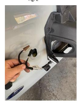
4. Remove stock plastic spare tire carrier. Using a 13mm socket, remove the 8 bolts on the outside perimeter of the stock plastic spare tire carrier (Figure D). SAVE THESE BOLTS, you will reuse them. Set the tire carrier aside to disassemble for the wiring harness. (Fig E)
