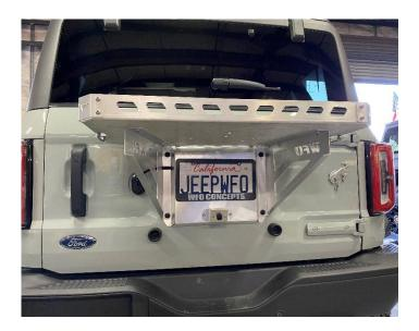
17. As an added bonus, if you want to leave the ice chest rack at home, simply un bolt the Qty. (4) support wing bolts from the tailgate and remove wings and rack together. Re bolt the (4) bolts back into the license plate mount and your good to go!
