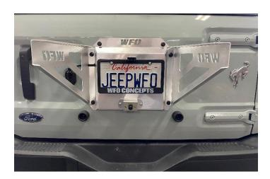
14. Locate your WFO 1401 Basket. If you have not previously assembled the basket, refer to those directions for assembly. Place the basket on the support wings. You will use Qty. (4) holes only. Look at the below picture for the holes. Fig. Q. Align the basket with the support wings till all 4 line up. You will use Qty (4) 1/2"-20 x 1/2" Button Allens, Qty. (8) 1/2" SS Washers, and Qty. (4) 1/4"-20 SS Nylock nuts.
