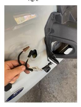
Remove stock plastic spare tire carrier. Using a 13mm socket, remove the 8 bolts on the outside perimeter of the stock plastic spare tire carrier (Figure D). SAVE THESE BOLTS, you will reuse them. Set the tire carrier aside to disassemble for the wiring harness. (Fig E)
