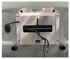
9. Take all 3 camera mount pieces. Start by sliding the pinch plate over the camera, with the Pem nuts facing away from the lens of the camera. Fig. M. Place the camera in the main mount, make sure the wire plug is pointing down out of the bracket. Slip the outer cover over everything. And last take the Qty. (2) #10-32 Button head allen's and thread them into the pinch ring. Fig. N
