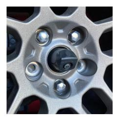
Using a 7/8" socket and impact gun, remove the 3 lug nuts for your spare tire. Remove tire and set aside.
