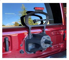
7. Install your new rack on the stock spare tire mount and tighten with the 3 previously removed lug nuts.
