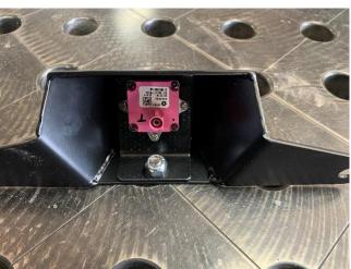
• Step 12) Hook the camera wire back up to the camera and install with 2 more factory bolts. Tuck wires gently behind license plate mount. (Figure L)
