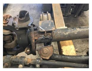
b. After the stock trackbar mount is off, cut the front section of the bump pad legs so they are flush with the top of the bump pad.
