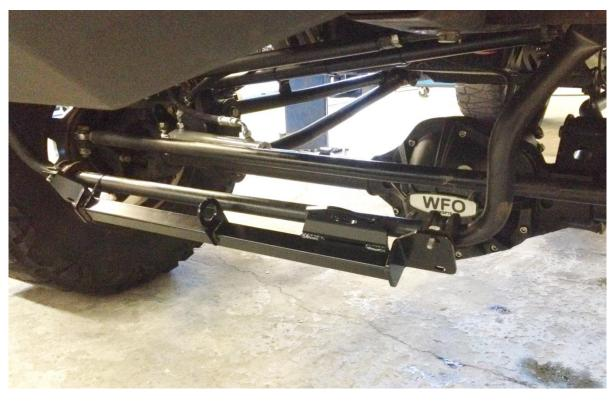
4.) Center the pitman arm stud in the hole of the steering box brace and install the bearing using the 7/16"-14 x 1.5" long bolts provided in the kit. It is recommended to lightly coat the pitman arm stud with grease prior to assembly. (This picture shows the brace installed without the swaybar)
