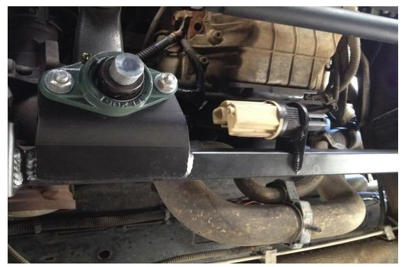
8.) We recommend Re-torquing the bolts after 100 miles of driving. Grease the bearing at normal chassis service intervals. Enjoy!
