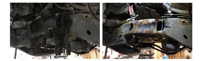
18) Remove as much as possible and grind clean in preparation for frame plates. \* Note the front crossmember in the picture below, you need to remove only the lower half of the crossmember. Especially if you are going to be running a sway bar, this mount needs to stay intact. \*
