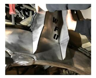
29) Before you completely weld the shock towers in place, you will need to locate the trackbar bracket on the driver side frame. The trackbar bracket will be placed inside the front of the driver side shock tower. Tack in place.
