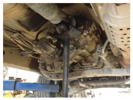
2.) Remove the 4 center factory transmission bolts using a 12mm socket.
