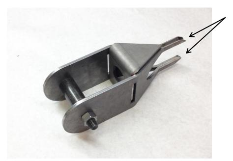
2.) **BEFORE WELDING**, slide your DOM into the clevis so it protrudes approximately  $\frac{1}{4}$ " into the clevis. This will give you plenty of space to weld around.
