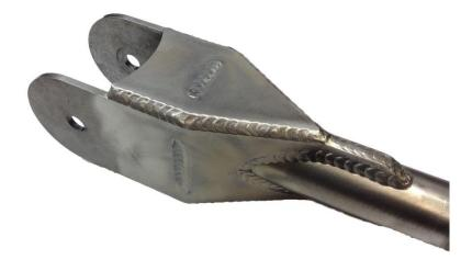
NOTE: When installing the clevis arms on the axle, the caps will be opposite of each other. For instance, the upper links should have the cap on the top side and the lower links will have the cap on the bottom side. This is for clearance issues with the factory axle bracket during cycling of the suspension. Otherwise, the clevis arms will hit the factory axle bracket.
